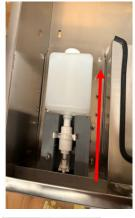
**Step 2:** To remove the soap dispenser slide it in an upwards direction.
