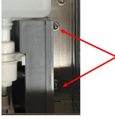
Step 1: Loosen the left and right fixing nuts.
